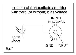
Some amplifiers only have a fixed bias voltage or the bias cannot be trimmed to near zero. In this case it is required to draw the ground level (which is not available on the input jack) from other sources, e.g. the output jack, special connectors or even from the housing. Please refer to the amplifier's manual and figure 2.
