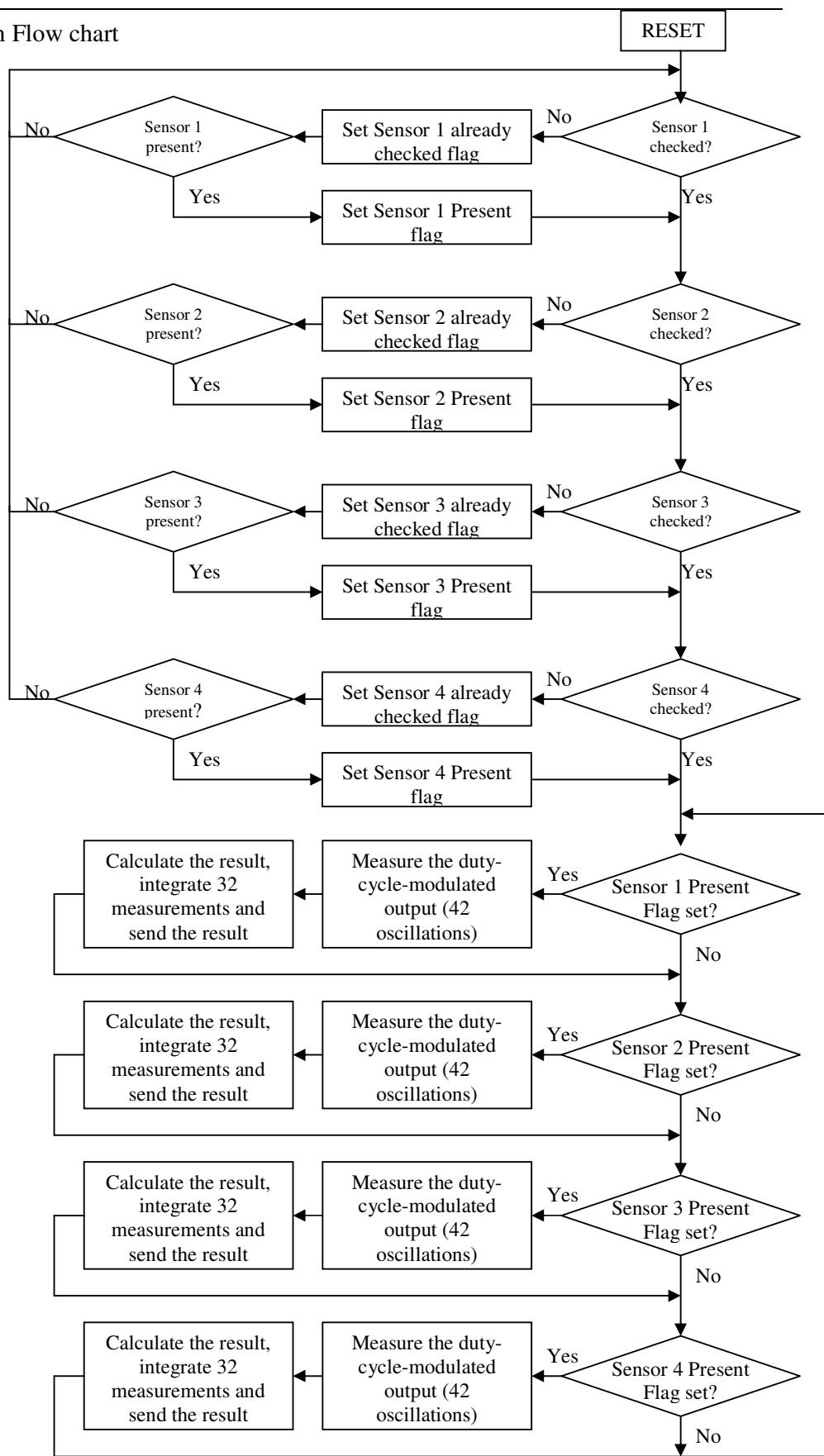
The measurement routine is based on a free running 16-bit timer TMR1. The counting frequency is 1 MHz. The flowchart of the measurement routine is shown on the figure:
